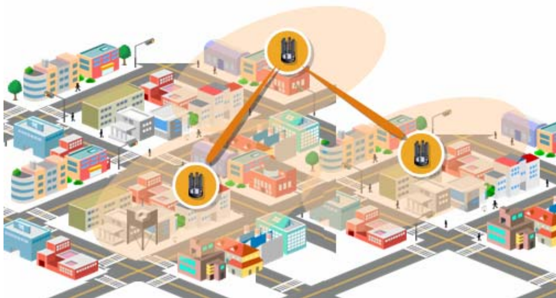
Figure 3.11 Self Backhaul Configuration
