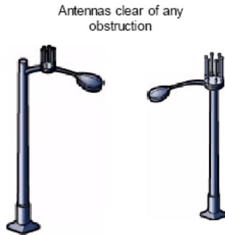
Figure 3.1 Example Mounting Locations on a Streetlight
