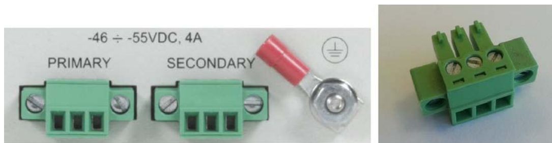
Figure 4-34: IDU-DT6 power connectors, grounding lug and power plug.
