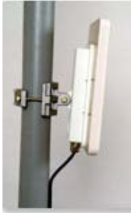
Figure 4-14: ODU with integrated Flat Panel antenna
