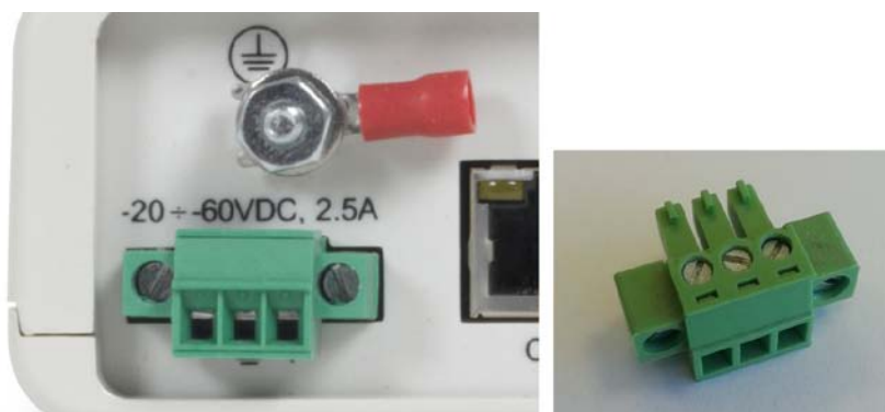
Figure 4-37: IDU-NetStream DT power connector, grounding lug and power plug
