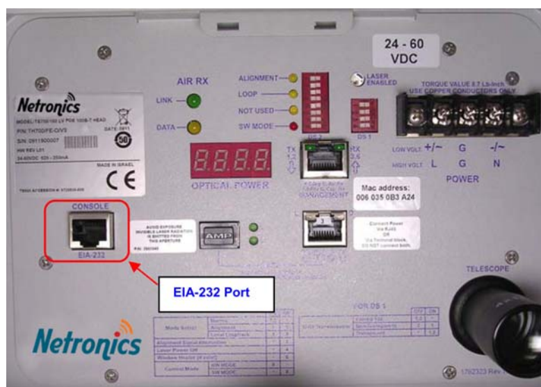
Figure 4: Connecting the RS-232 cable – NL100-880
