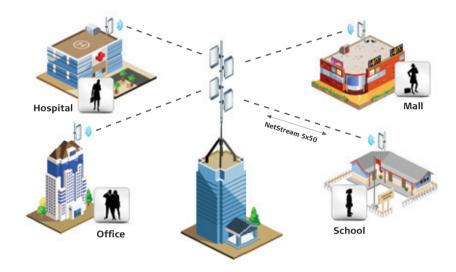
Leveraging from Netronics proprietary air interface, coupled with advanced built-in OFDM, MIMO and Diversity technologies, NetStream 5x50 delivers optimal performance and unequalled robustness in sub-6 GHz bands. The high-capacity solution can be deployed in various topologies including point-to-point, cascading and multiple point to point, and support collocation with other NetStream radios utilizing Hub Site Synchronization (HSS) functionality.
