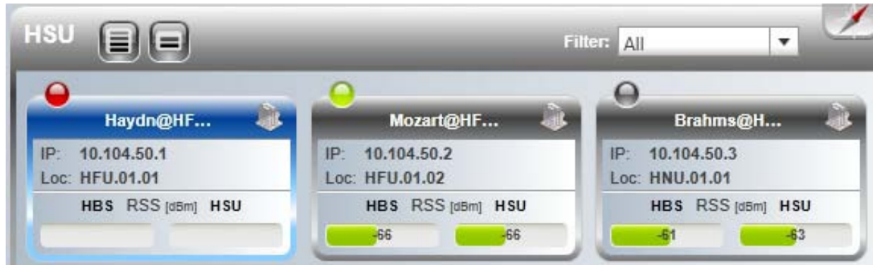
Figure 6-18: Unit 10.105.50.1 is down; unit 10.104.50.2 is available and 10.104.50.3 is not registered
