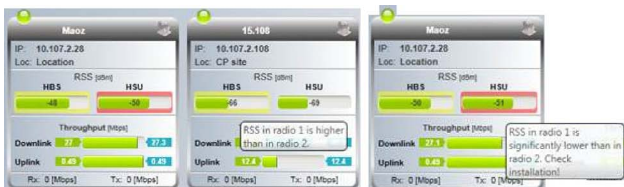
Figure 4-26: HSU status boxes - detail, indicating problems
