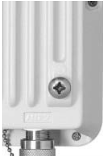
Figure 3-29: HBS: Grounding lug
